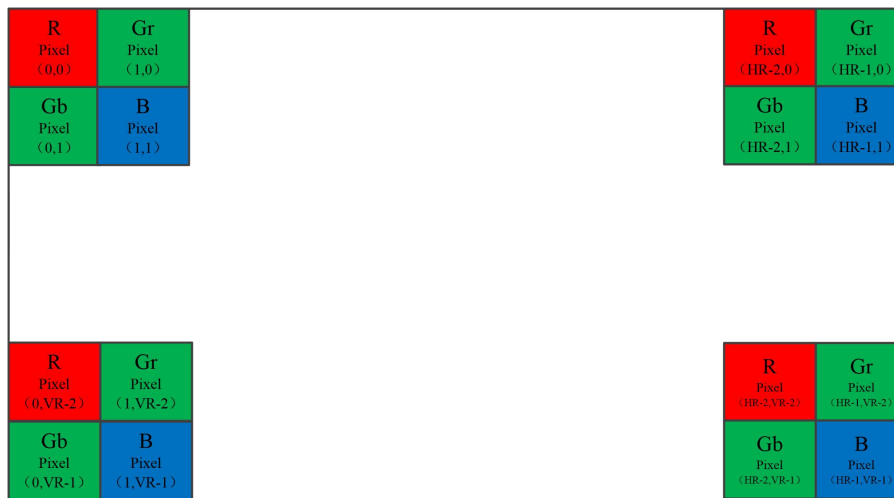
Fig. 4 Camera Bayer Arrangement
