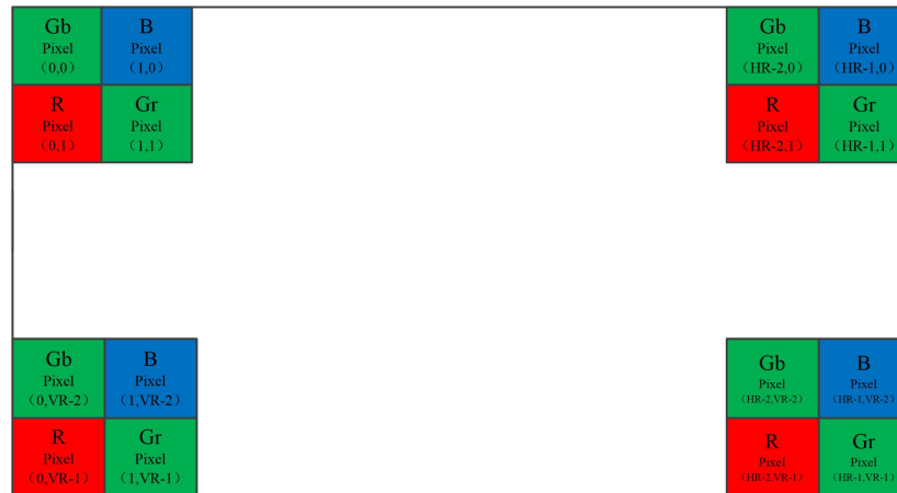
Fig.4 Camera Bayer Arrangement
