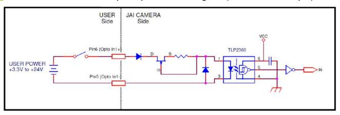
**Caution:** Check the recommended reference examples for proper wiring. If Opto In 1 (Opto In +/ Opto In -) and Opto Common are connected reversely, the camera may be damaged.
