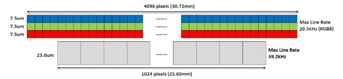
JAI's ImageScalingMode applies an interpolation algorithm to the pixels on the RGB sensors to create larger virtual pixels that aren't limited to multiples of the base pixel size. By using ImageScalingMode in conjunction with the ROI function, the pixel size and the FOV of the RGB channels can be normalized with those of the SWIR channel. At the same time, the line rate of the RGB channels can be increased, allowing for the RGB and SWIR channels to be synchronized at a faster line rate.
